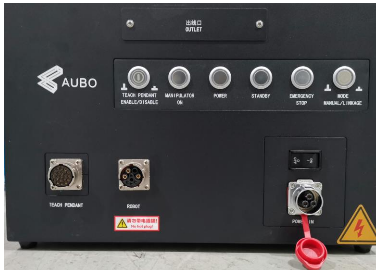
Figure 7-2 Front panel of the control box
