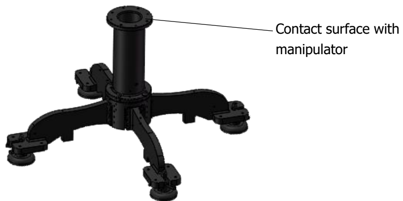
Figure 6-3 Diagram of manipulator base structure
