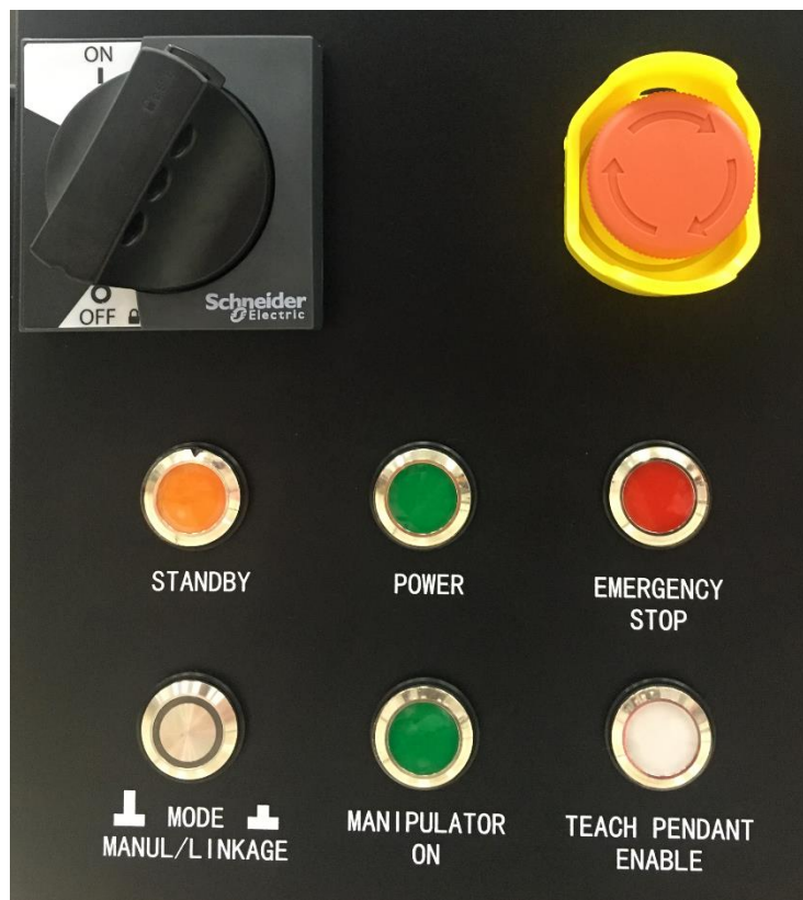
Figure 7-2 Schematic diagram of the front panel of the control box
